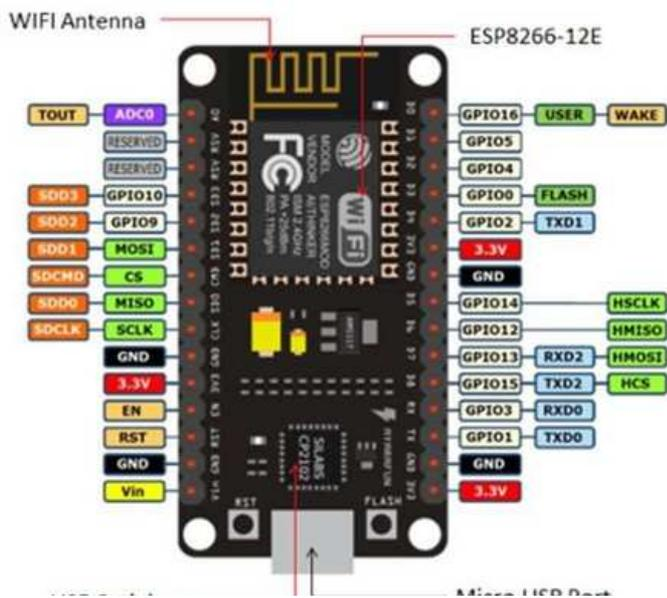
The NodeMCU\_ESP8266 is basically a WIFI module integrated with a Microcontroller, which makes it a very useful device for this project,
